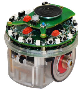
Figure 2. The e-puck is a differential drive robot with a diameter of 75 mm and is equipped with a variety of sensors and actuators, such as a color camera, infrared proximity sensors, a loudspeaker, 3 microphones, and two wheels. Our e-pucks are also equipped with a range & bearing board that allows for inter-robot communication.
