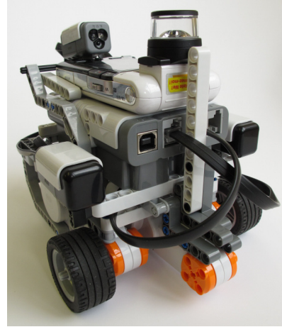
Figure 3. The LEGO ® MINDSTORMS ® NXT robot used for the experiments presented here. The robot is equipped with an on-board omnidirectional video camera (above the NXT brick) a gyroscopic sensor and an acceleration sensor (pictured to the left and right above the wheels). For locomotion, the robot uses two active wheels (seen at the front) and a dummy castor (not visible in the picture).
