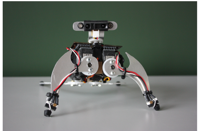
Figure 1. The walking robot Hodgkin with four legs, five motors and an "artificial brain" of 19 neurons.
